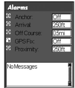
At the bottom of the display is a field that will display information about all alarms that have been triggered since the eXplorist was last turned on.
